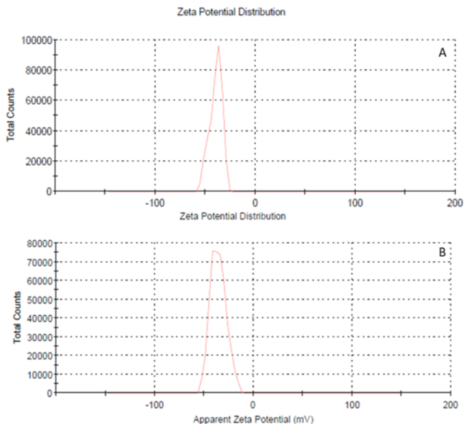
Figure 3. Zeta potential distribution of the final formulations A. F3 and B. F4 by Zetasizer, Malvern Instruments.
